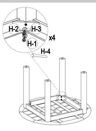
Place Table Top Panel (A) upside down on a padded non - marring surface. Insert bolt on Leg (B) through predrilled holes in corner of apron. Secure bolts with Flat Washers (H-3), Spring Washers (H-2) and Hexagon Nuts (H-1), stacking the hardware in the order as shown. Loosely install hardware on both bolts. Fully tighten using Open Wrench (H-4) after all hardware is installed. Repeat for remaining Legs (B).
